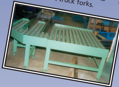
Special die table with slots for fork-lift truck forks.
